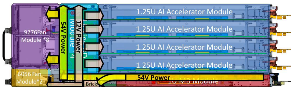
Figure 7. A side cross-sectional view of the Galaxy server.
